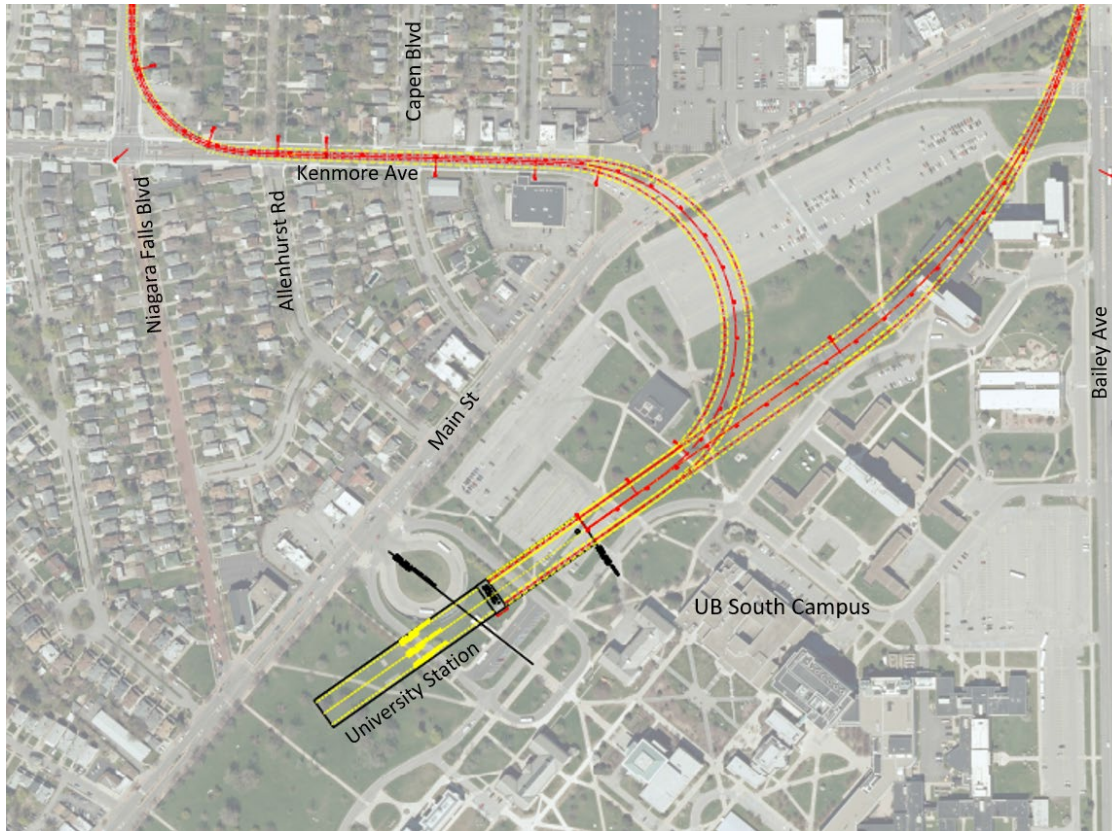
Figure 5: University Station / Bailey Avenue Curve
