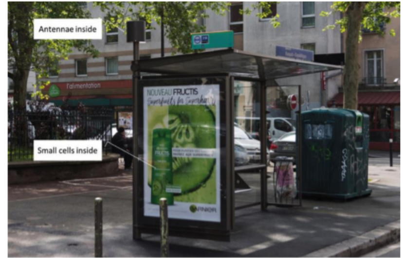
Figure 5-5: Small Cell technology incorporated into a bus stop shelter www.ict.illinois.edu
